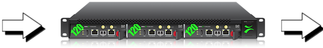
Figure 4.5: The ACC Unit with probe boards installed – Direction of Air Flow
